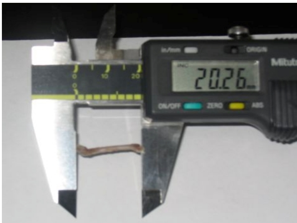
Figure 1 Length measurements were obtained by placing the outside measuring faces of the caliper proximally at the tip of the humeral head and distally at the groove lateral to the medial condyle (shown above). Width measurements (medial-lateral and anterior-posterior) were taken at 50% of the length of the humerus (not pictured).
