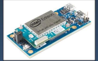
Having a multitude of GPIO pins was essential in the decision to use the Intel Edison. Each subsystem of the controller requires signals from the embedded system in order to change its behavior based on a desired function. The GPIO pins allow for this type of communication by using the GPIO pins for HIGH/LOW signals and specific functions such as Inter-Integrated Circuit (I2C) communication for accessing additional hardware
