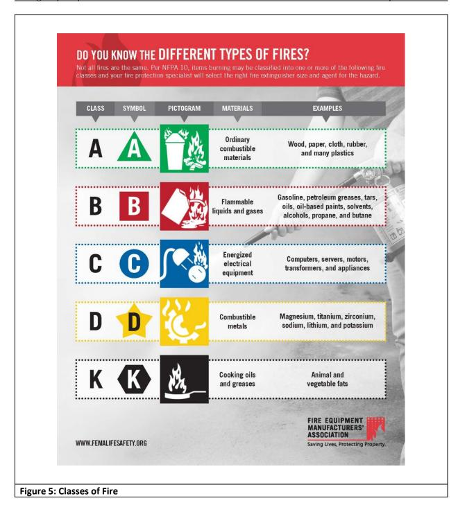
An attempt to extinguish a fire with just any extinguisher may have undesirable effects. To prevent this, one should become familiar with the various types of extinguishers found on campus. All extinguishers should be marked with letters or pictograms depicting the extinguisher's classification.
