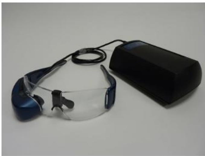
Fig. 2 Virtual reality glasses (VRG) and processing unit. Note the display screen in the right lens, which is placed below the patient's line of sight
