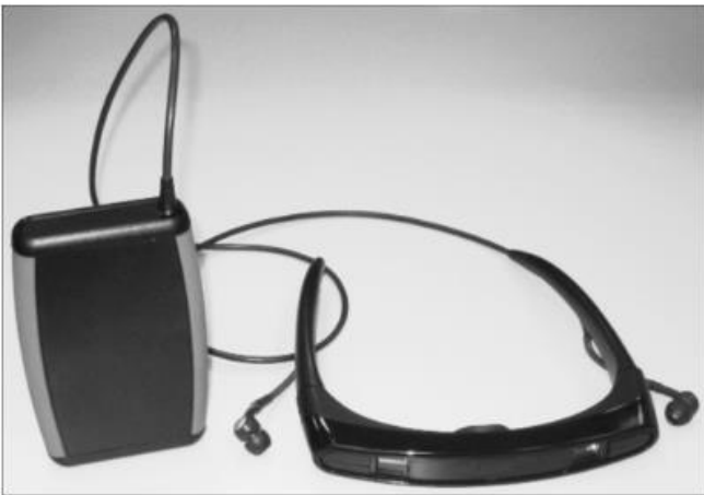
Figure 1. Virtual (augmented) reality goggles used in this study containing built-in LCD screen, which projects floor tiles when subjects are moving, and earphones that sound step-matched cue as determined by connected sensor strapped at belt.
